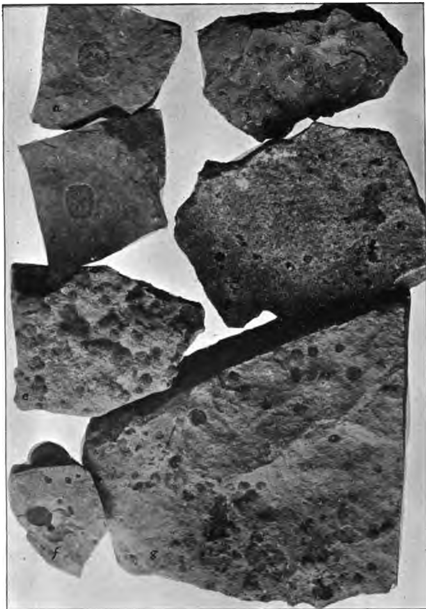
Cordierite-hornfels in which cordierite is replaced by chlorite nodules, forming the "spotted slate" (spilosite) of the slopes of Rocky Hill, Sourland and Round Mountains; a, b, c, f , from old copper mine near Griggstown; d , \frac{3}{4} mile south of mine, chlorite nodules very small, black tourmaline crystals prominent; e , west side of Round Mountain, weathered surface with projecting nodules; g , \frac{1}{4} mile south of Round Mountain, \frac{1}{8} mile east of Rowland's Mills. Three-fourths natural size.
